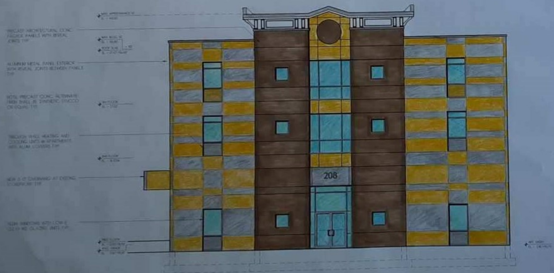
(A1) PROPOSED NORTHEAST BLDG. ELEVATION SCALE: 3/8" = 1'-0"
